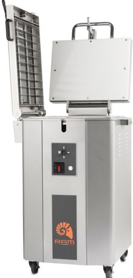
The working cycle provides cutting by manual closing of the interchangeable side grid and operating by the joystick to raise and lower the pressing plate. Furthermore, it offers the possibility to make the only pressing by joystick and closing of top cover. The DSSGRID model allows to divide medium/strong dough by the lower knives.
