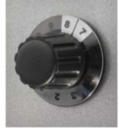
Single/Three phases version with Inverter to change the belts and cylinders' speed
